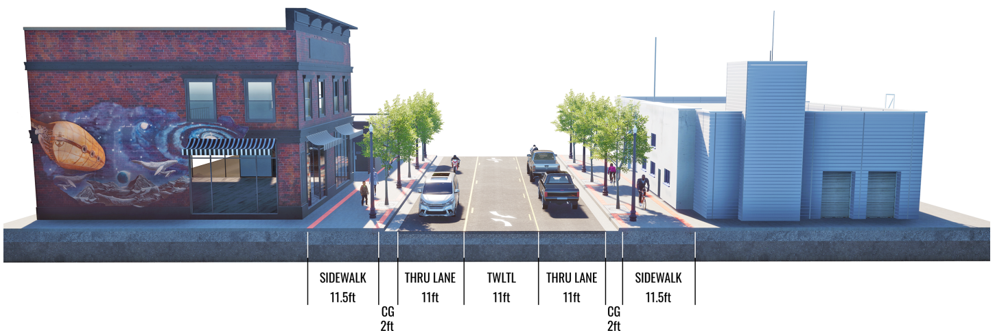
Fig. 12 - SR 37 Typical Section
