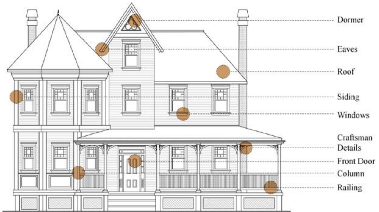
Figure 5.15: Queen Anne Facade Features
